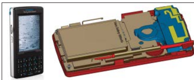
▲ Fig. 5 Full phone model containing phone plastics (red and blue) and metallic parts (copper and gold).
