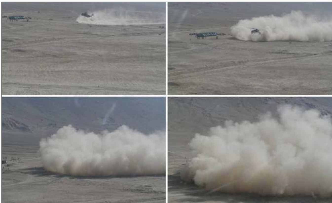
▲ Fig. 1 Dust clouds completely engulfing a landing helicopter.
